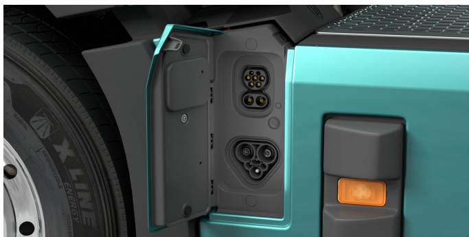
Megawatt Charging System (MCS) et Combined Charging System (CCS2).
